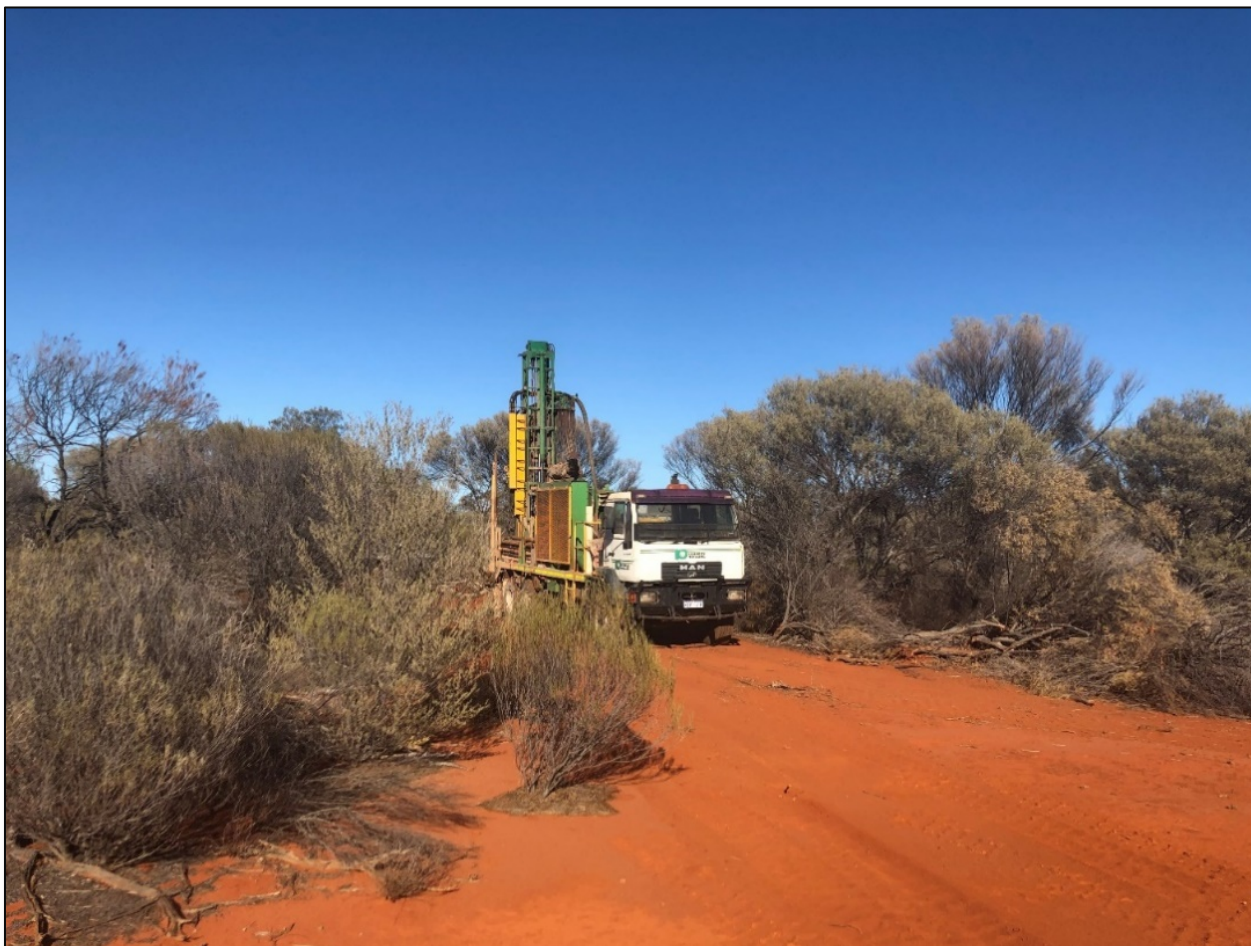
Figure 5: Aircore rig in action at the Laverton South Project
