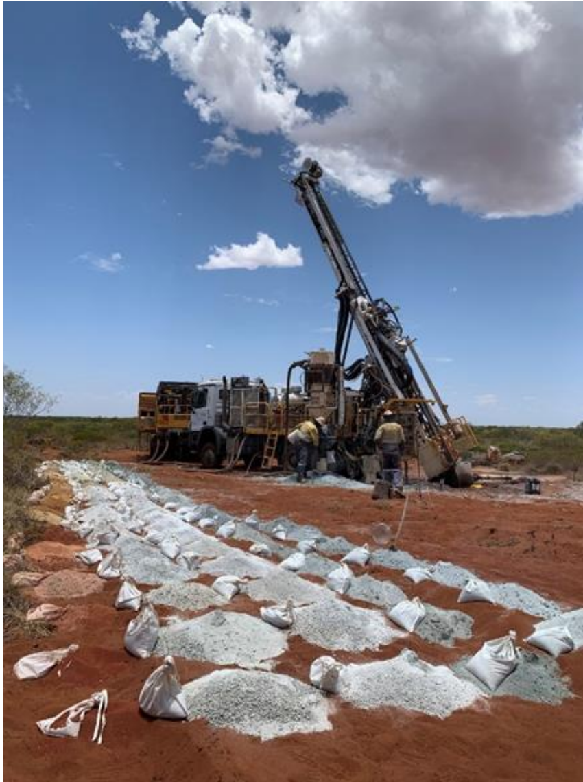
Photo 2: Strike Drilling T450 Aircore/Reverse Circulation Rig
