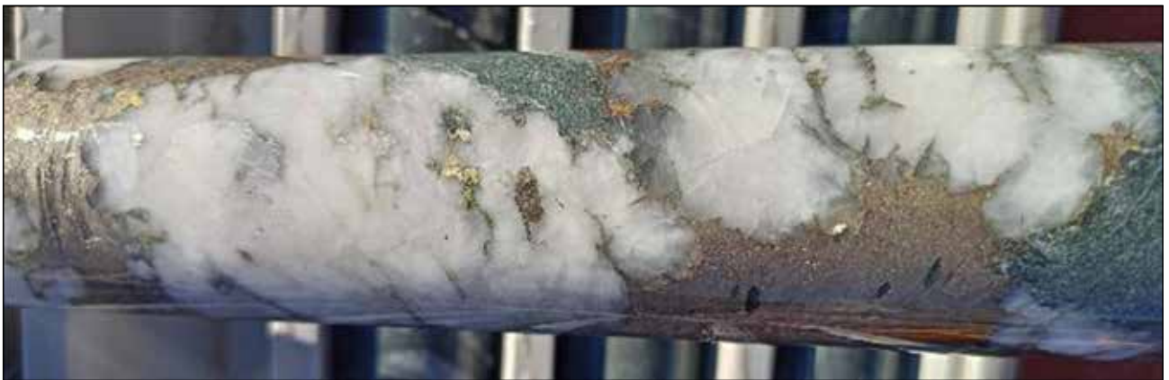
Figure 11: FMDD0047 -231m, sulphide bearing quartz vein with pyrrhotite, pyrite, arsenopyrite and chalcopyrite hosted within andesite volcanics.
