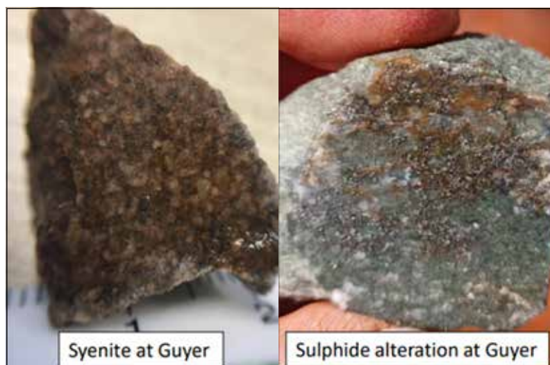
Figure 25: Examples of a favourable syenite intrusion and sulphide altered andesite intersected by AC drilling in the Guyer Target Area.
