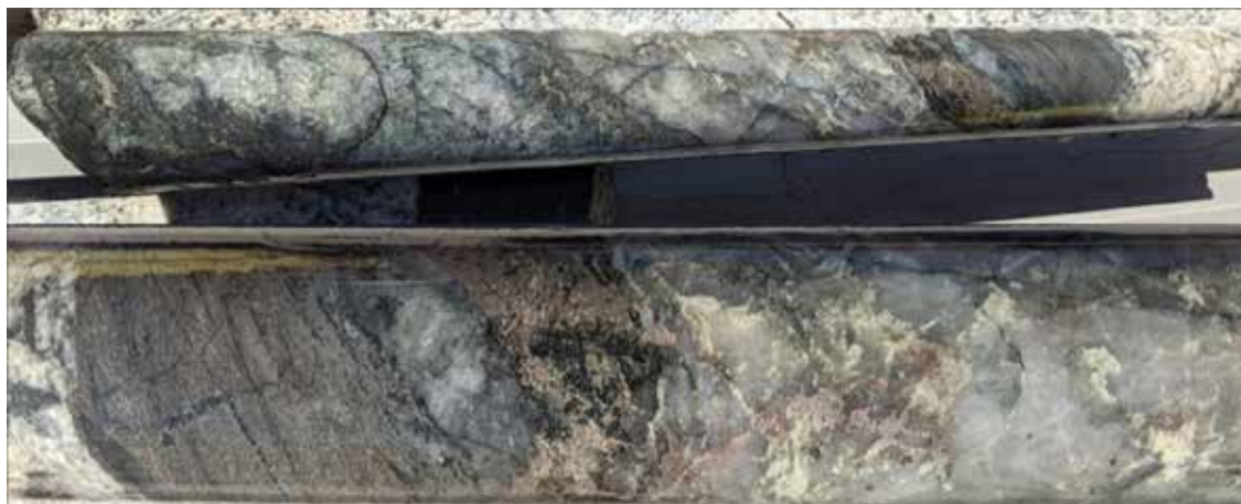
Figure 21: FMDD0032 -116m Sulphide bearing lode structure.
