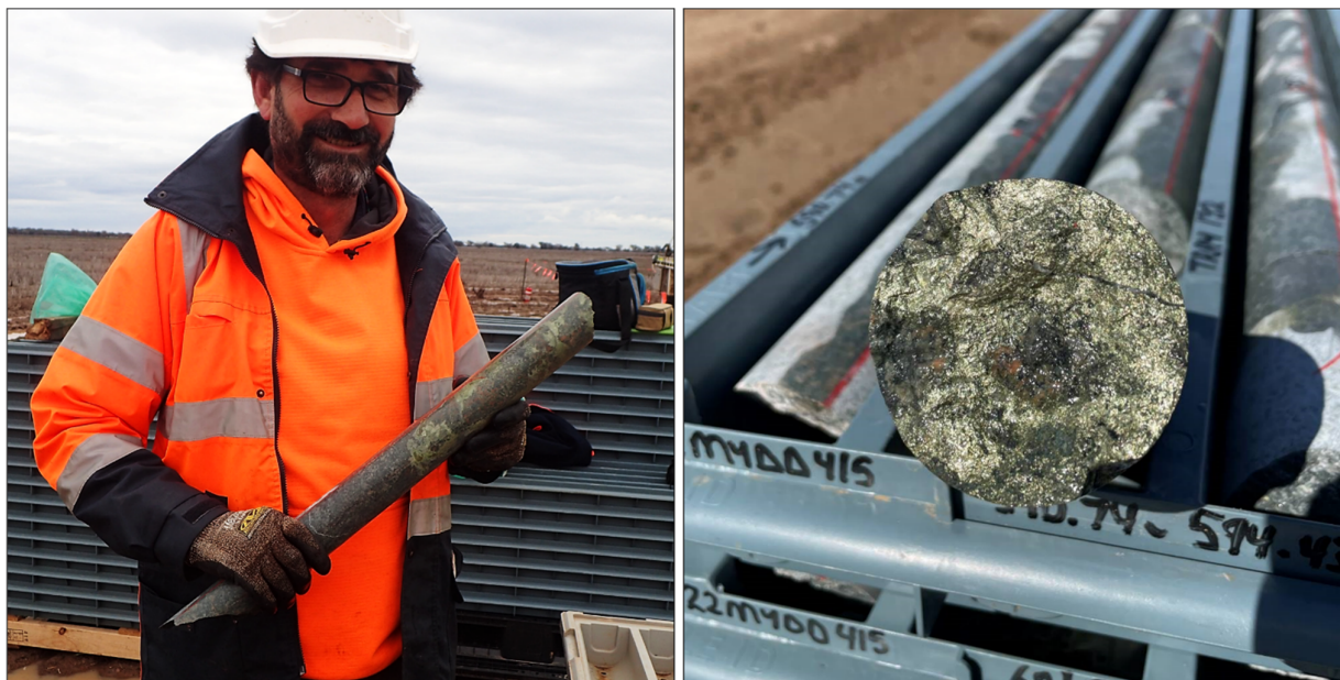
Figure 5. Magmatic Resources' Exploration Manager, Steven Oxenburgh, holding core with abundant breccia-hosted chalcopyrite (yellow) from 588m down hole in 22MYDD415 (left); and cross section of core from 591.6m down hole displaying semi-massive, breccia hosted chalcopyrite from 22MYDD415 (right).
