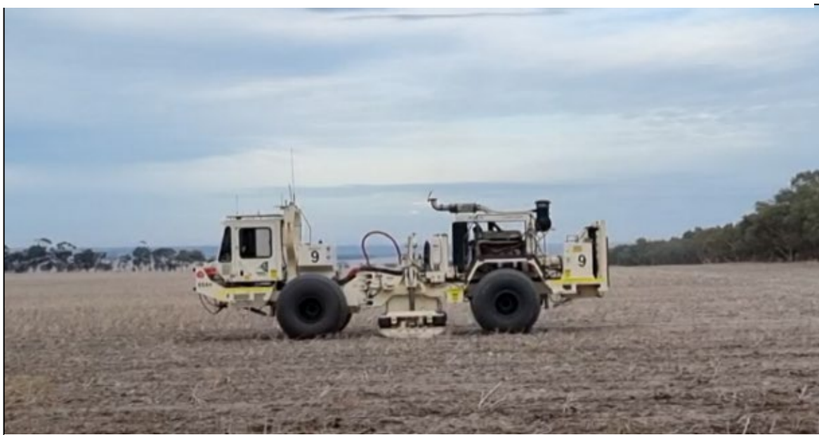
Figure 8: Bookara 3D Seismic Vibroseis seismic acquisition vehicle near Mt Horner
