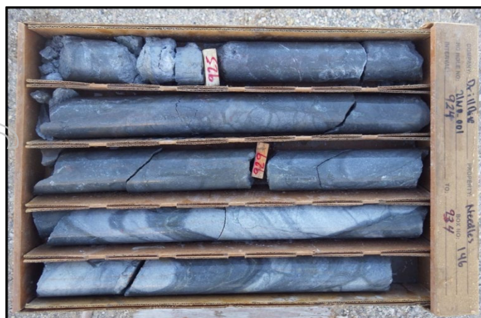
Figure 5. Core photo from 924ft to 934ft (281.6m to 284.7m) in hole 21ND_001 showing silicified and propylitically altered andesites containing disseminated and vein-hosted pyrite (grey).
