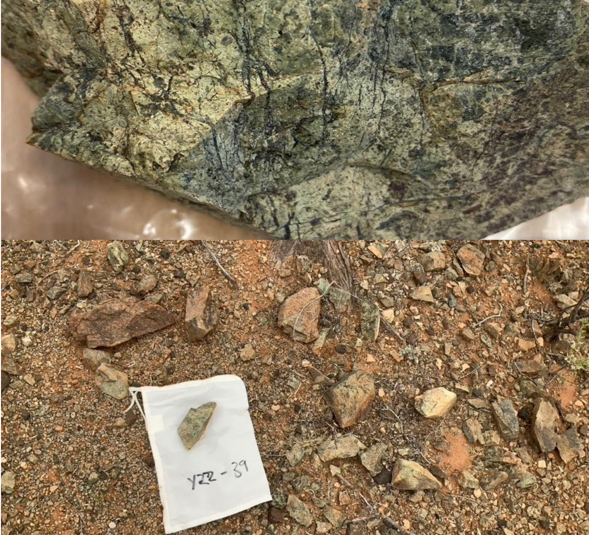
Picture 2: Yinnetharra (WCN 100%) REE/Li project, sample YZZ39 which is highly anomalous in REE's with a grade of 615ppm TREO, and thought to be proximal or near a stronger mineralised source. YZZ39 is proximal to a thorium anomaly.
