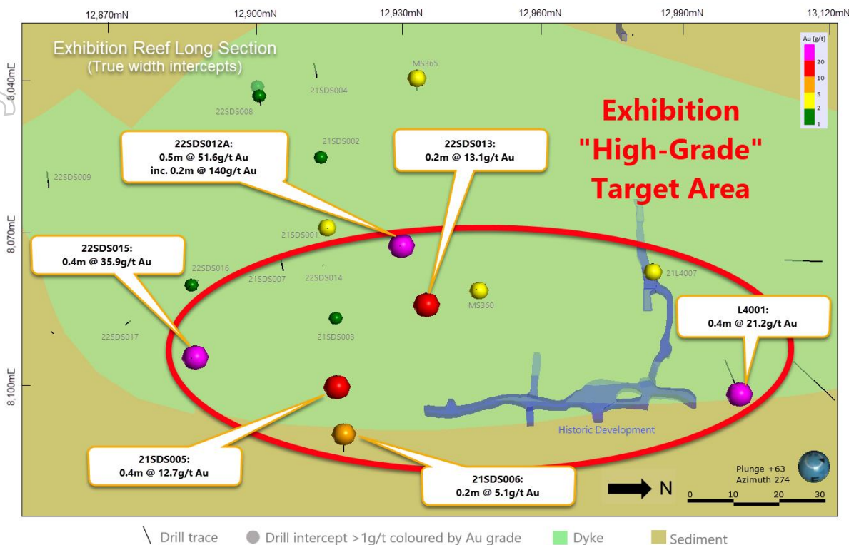
Figure 6: Exhibition Reef long section plan view showing the Morning Star host dyke (green), historic mining and mine development (blue) and all historic & current drill hole traces with pierce point intersections. The “high-grade” target area with 100 metres of strike and 40 metres across strike extent is defined by drill intercept pierce points shown.
