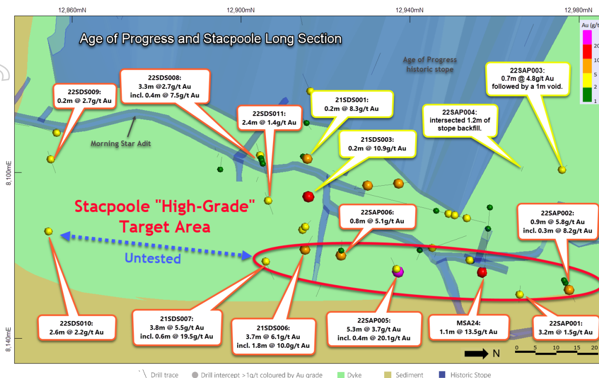
Figure 7: Long section view through the Stacpool Reef showing current and historic true width drill intersection pierce points, the limited historic stoping on the Age of Progress Reef and the potential “high-grade” target area along the eastern edge of the dyke where the Stacpool and Age of Progress Reef come together (refer Figure 2). Stacpool Reef intersections outlined in orange and Age of Progress intersections outlined in yellow.
