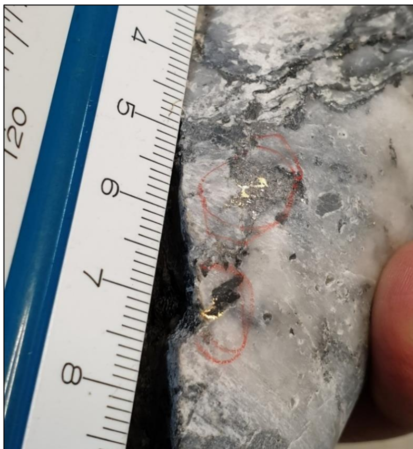
Figure 10: Visible gold within an interval that assayed 0.25 metres at 972g/t gold in diamond drill hole 22GZL9016 testing the Gap Zone at the Morning Star Gold Mine.
