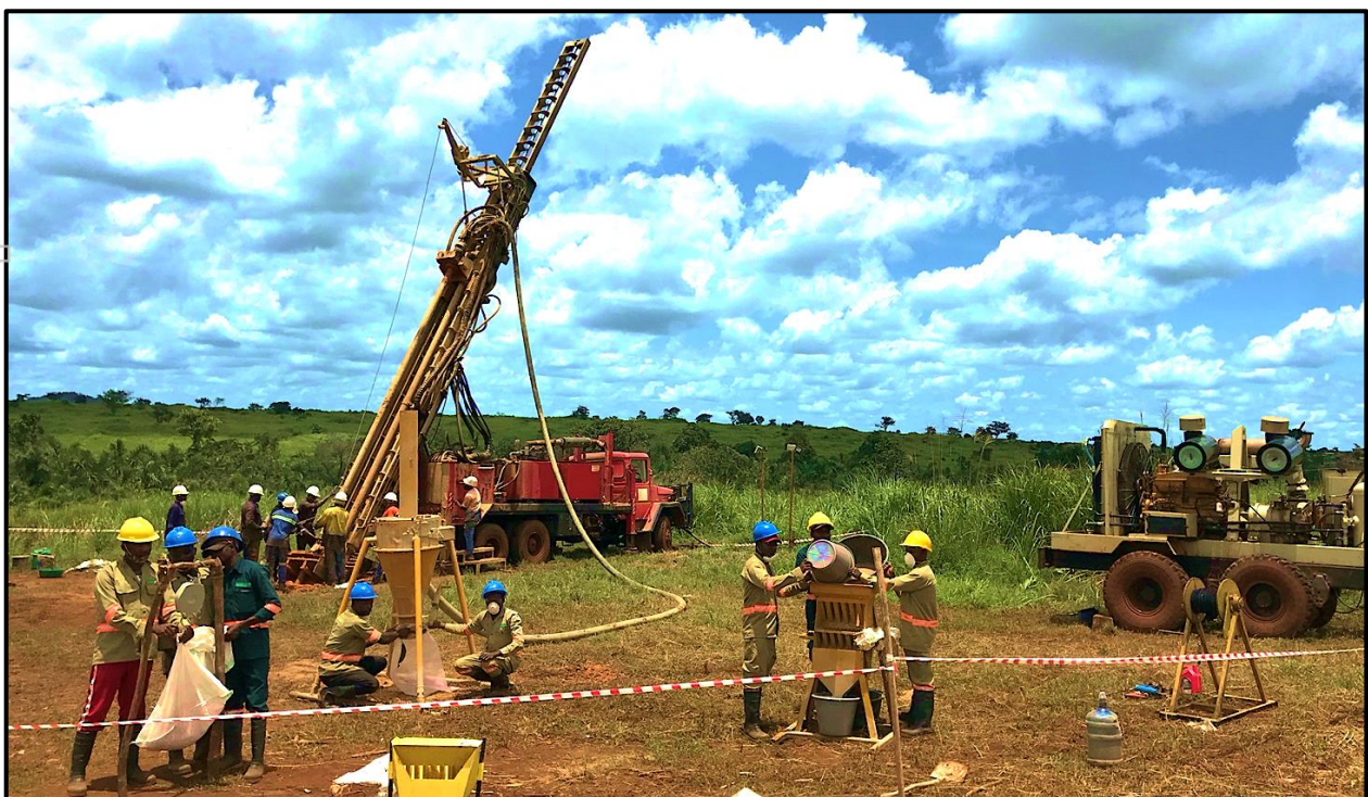
Figure 5 - Photo of RC Drilling at Kebigada South-East.
