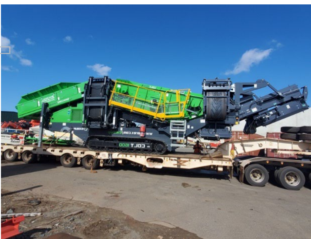
Figures (1.3.1) & (1.3.2): Scalper and Radial Stacker Conveyor Units mobilising to Butcherbird
