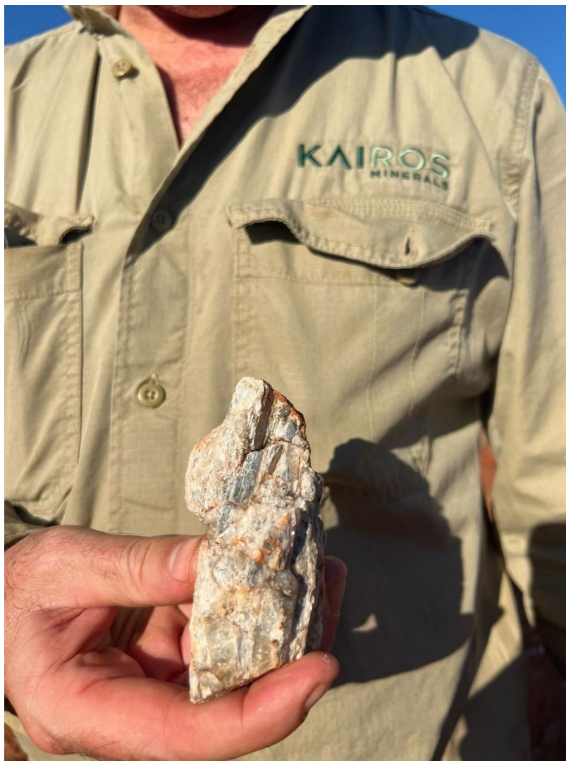
Figure 10. Kairos Geologist Campbell Watts holding a piece of spodumene-bearing pegmatite (MYR393 – 1.91% Li 2 O) discovered at 'Lucky Sump' during routine earth moving activities.
