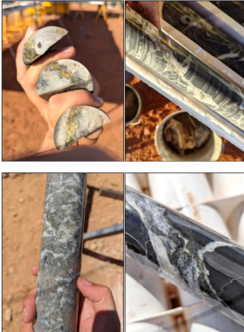
Photo's 1: Clockwise from top left – Chalcopyrite (cp) in quartz veining, pyrite (py) ± cp along discordant quartz-carbonate veins selvage, py ± cp veining with quartz-carbonate veining in siltstone, and fine disseminated pyrite in altered and brecciated Dolerite near apex zone.
