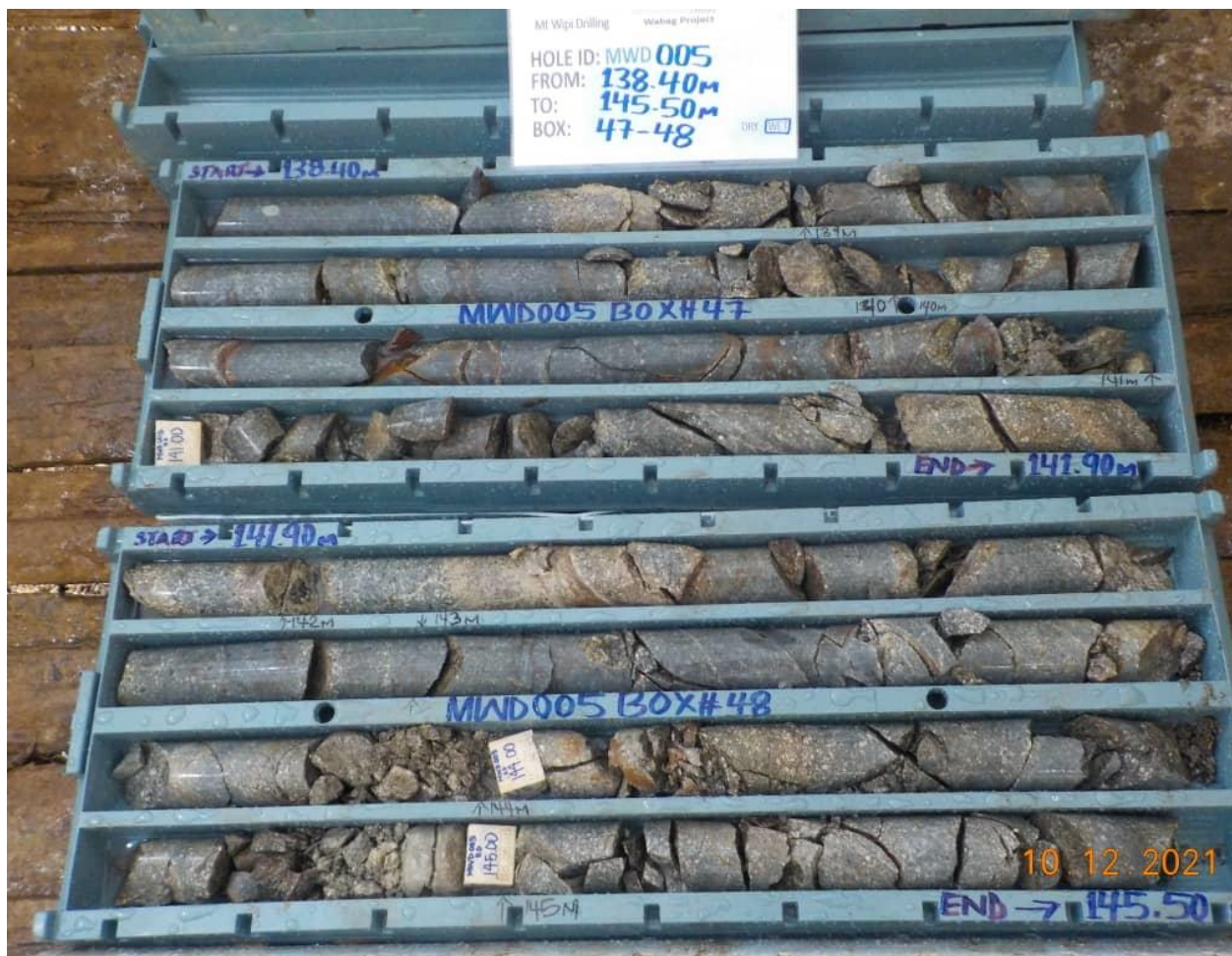
FIGURE 1. CORE FROM MWD005 WHERE THE 11.7G/T GOLD ASSAY WAS RECORDED BETWEEN 144 TO 145M
