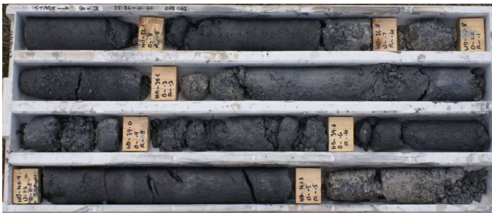
Figure 3: Original core from OAD002, (containing 1.7m @ 16.65% TGC from 39.60m), prior to sampling and resampling for the new testwork to feed into the updated scoping study
