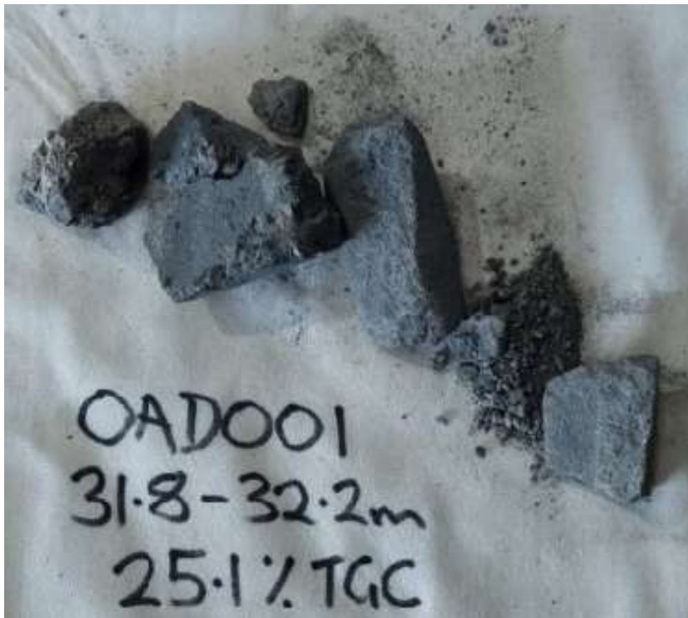
Figure 2: High-grade diamond drill core fragments from OAD001 – resampled for revised testwork
