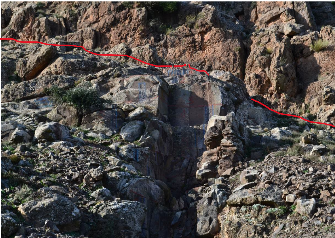
Figure 03 – KEL Trenching Showing Phosphate Mineralisation (Lower Layer) and Dolomitic Limestone Overburden
