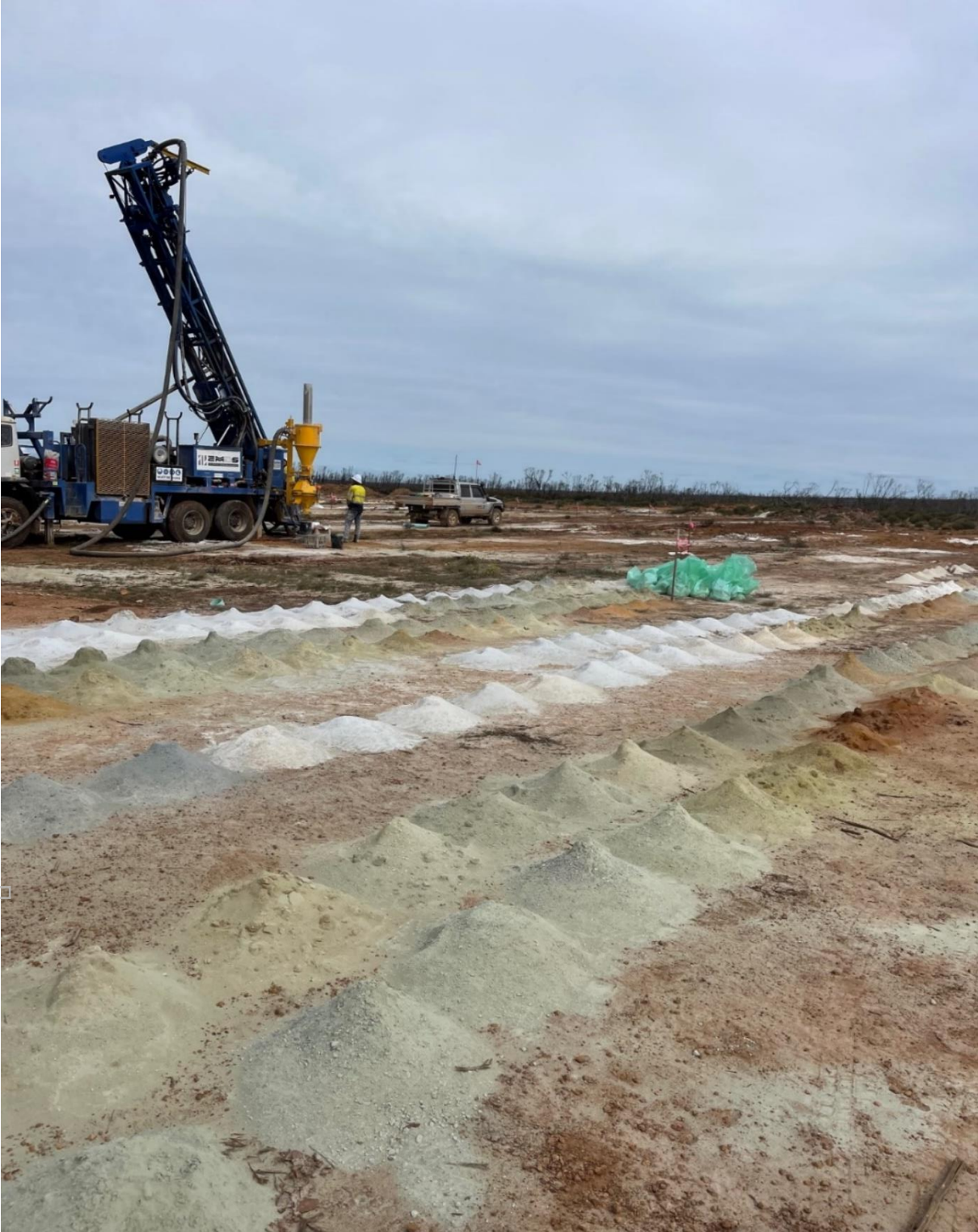
Figure 4: Infill RC Drilling at Kat Gap
