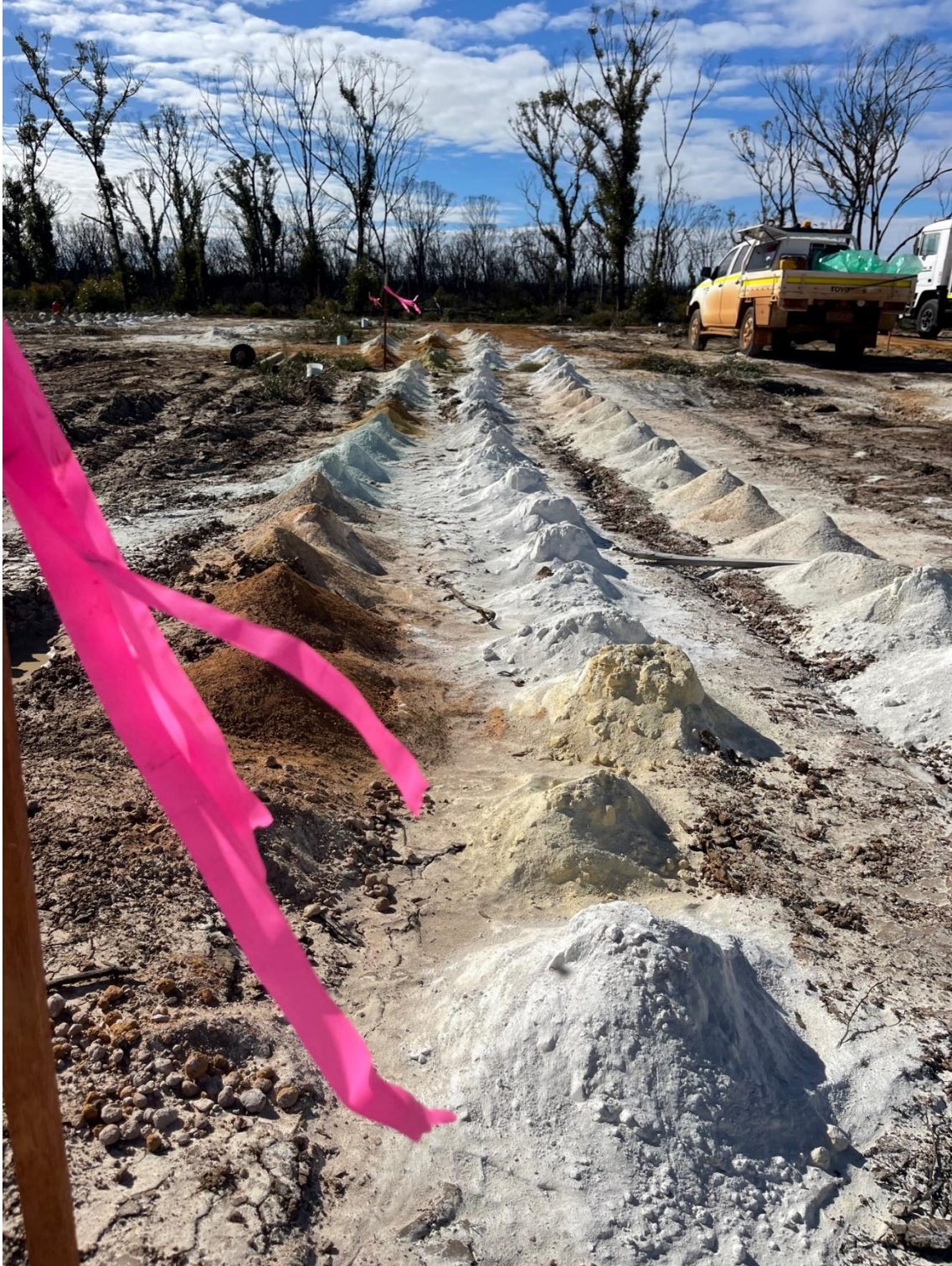
Figure 3: Infill RC Drilling at Kat Gap
