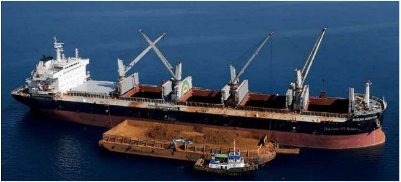
Figure 27 Typical Geared Bulk Carriers for Nickel Ore export
