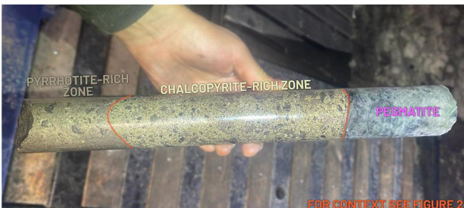
Figure 1: Core Photo of Chalcopyrite rich zone from mineralised interval in KNI_ER003
