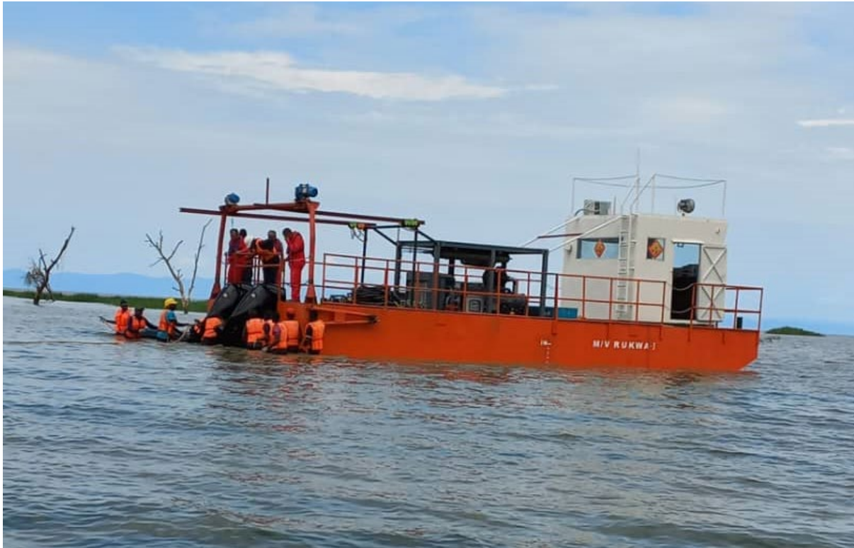
Figure 1 - 3D seismic source vessel at the conclusion of Phase 1 operations in Lake Rukwa
