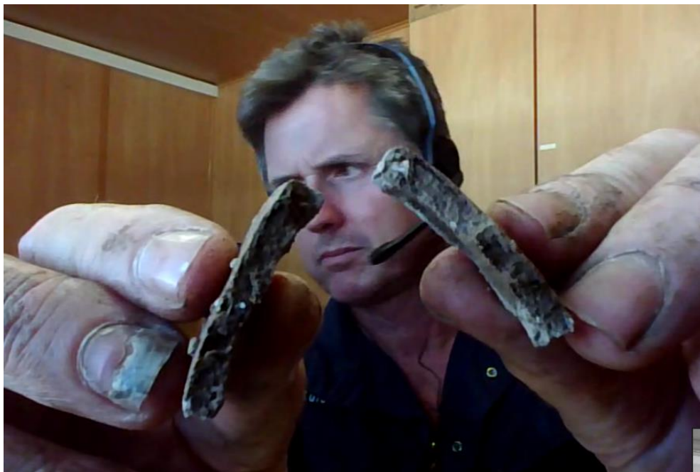
Figure 2 – Example of filter cake recovered from side wall cores
