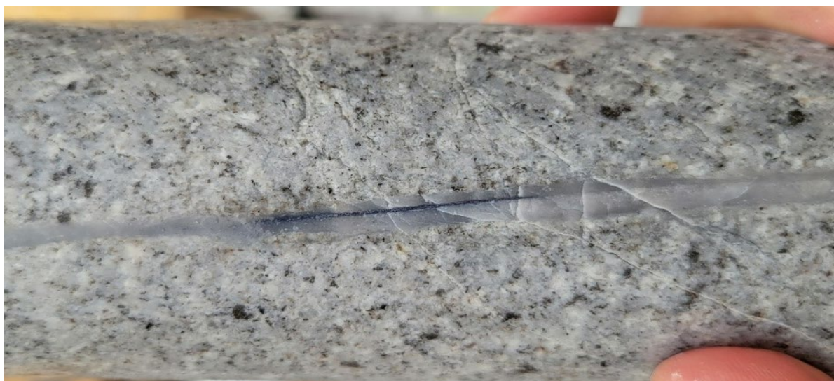
Figure 12: Molybdenite within quartz vein in drill core from WD22-01C at approx. 744.29m (2442ft).
