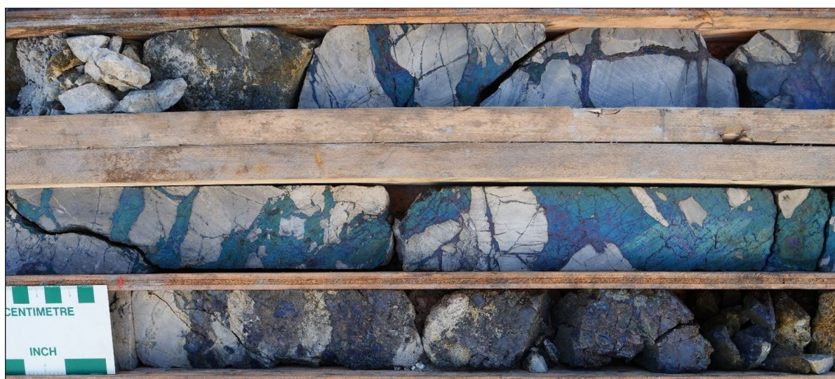
Figure 4: Massive and fracture-fill bornite and chalcocite from approx. 50m downhole in ST22-05.
