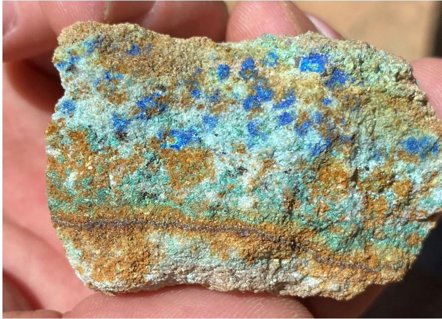
Figure 24: Coarsely disseminated copper oxides (in this case azurite – brilliant blue in colour) are widespread in outcrop throughout the Copper Warrior Project area.
