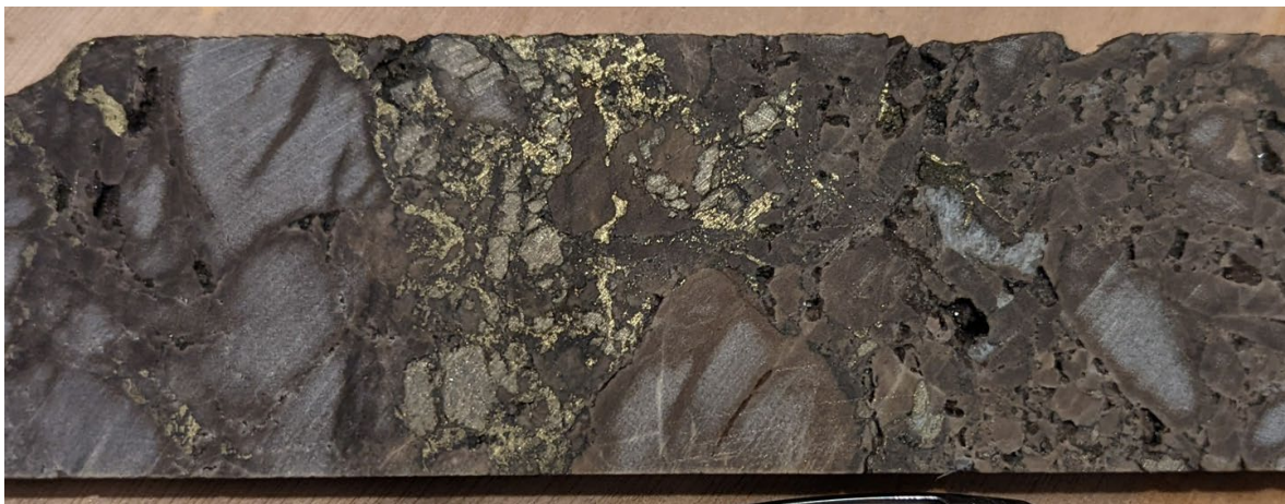
Figure 7: Chalcopyrite (copper sulphide) within ST22-10 drill core from 313m downhole.
