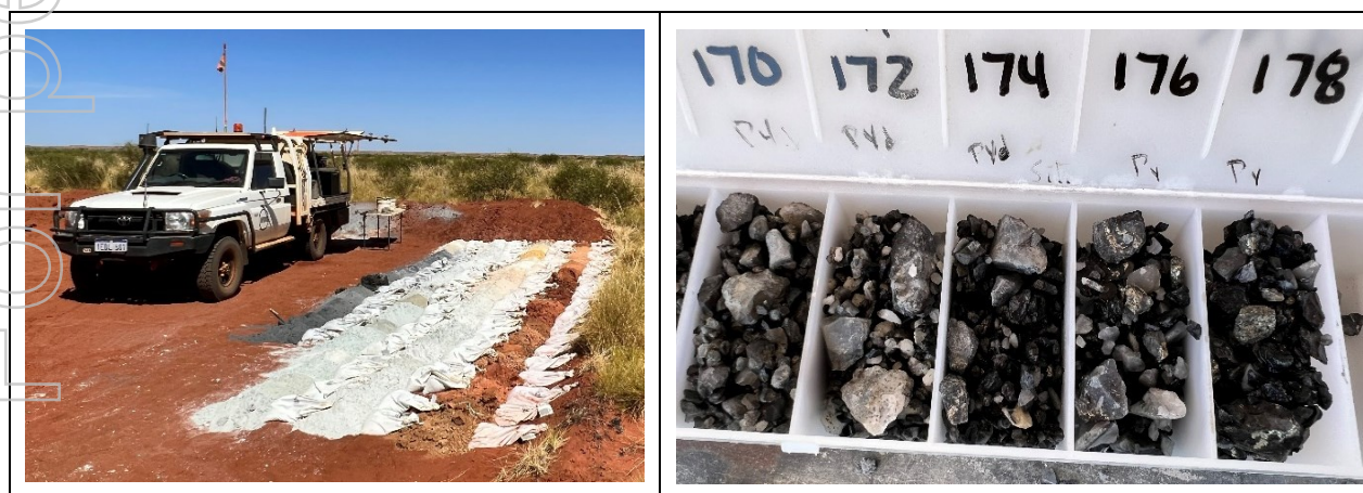
IMAGE 2: RC DRILLING SAMPLE BED AND PREPARATION
