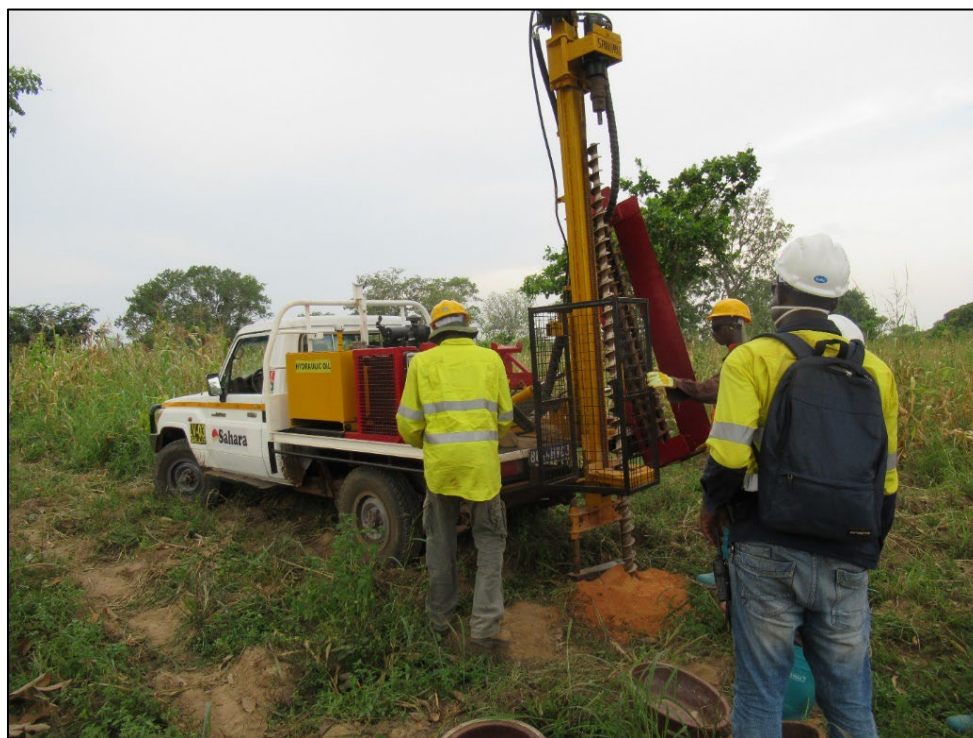
Figure 5: Auger rig drilling during phase 1 auger program
