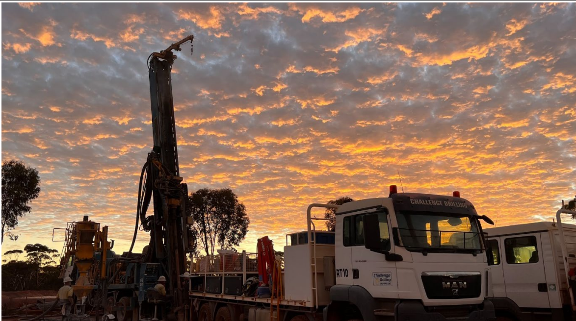
Image 1 – RC drilling at Hestia
