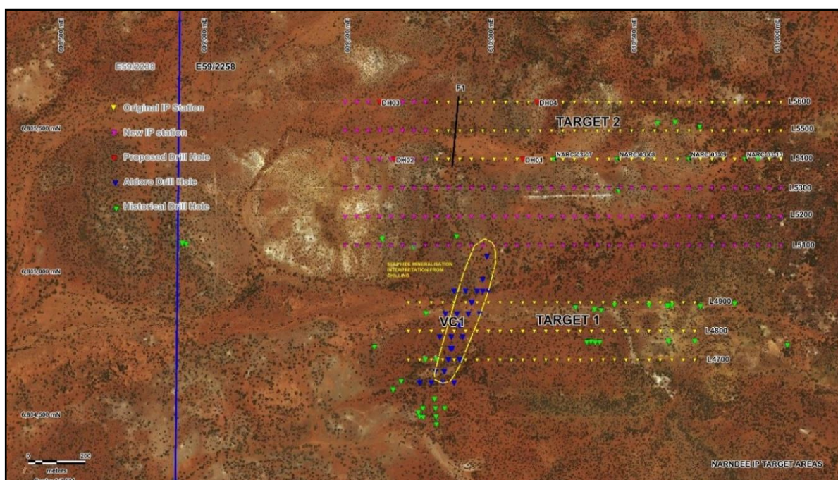
Figure 7: Location of the IP survey station/lines, all past drilling, VC1 interpreted mineralisation from drill intersections and the four proposed holes.
