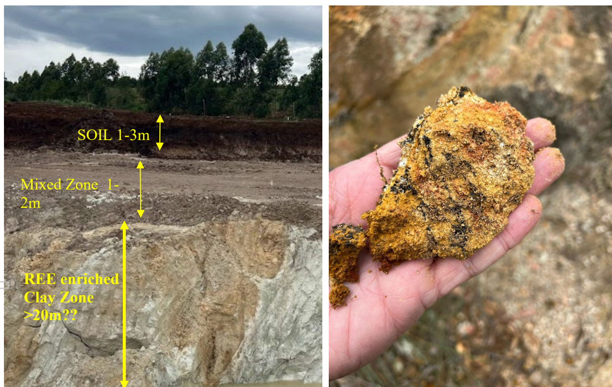
Figure 3. a) From Togni SA refractory clay mining pit at Capo do Mel (CDM) Project highlighting the thin soil horizon (approx. 1m this area) underlain by a mixed clay soil zone 1-2m thick and then a mineralised clay zone enriched in REE. b) Detail of REE enriched clay-zone sample from clay mining area on CDM Prospect. Note: the thicknesses of horizons may vary considerably across the project. REE mineralisation has been found in all zones.
