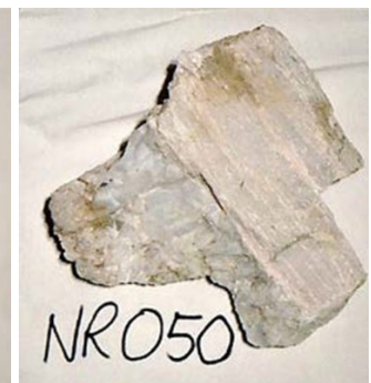
Figure 7: Quartz-spodumene-albite-muscovite rock. About 15% spodumene
