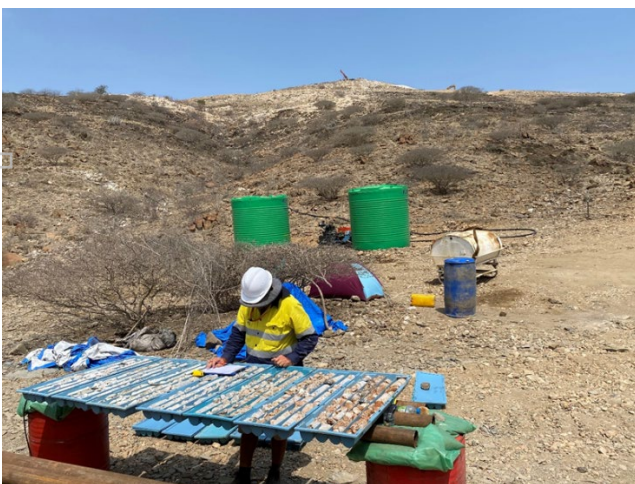
Figure 9: Core-trays laid-out on makeshift core rack at site. Note drill-rig in background on top of hill, set-up on drill-hole NDDH004. Geologist Neil Scholtz logging drill-core from NDDH004.
