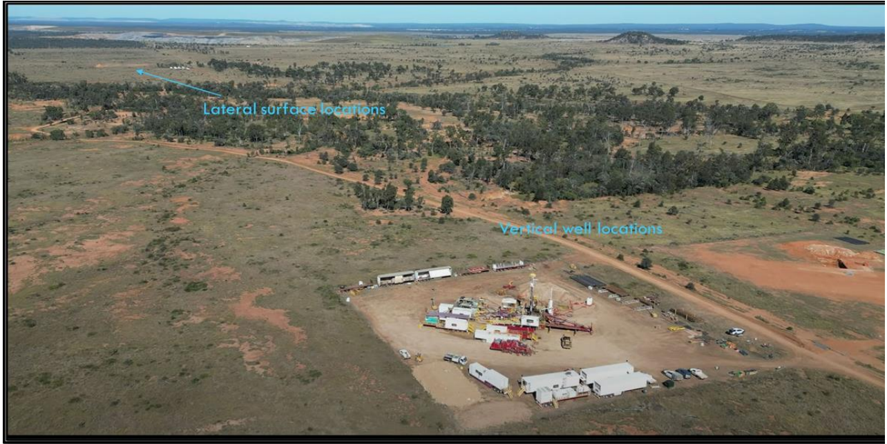
Figure 1 : Layout of Blu's Sapphire 5 vertical well (foreground) and location of the Sapphire 5L pilot wells (with the Isaac Plains Coal Mine) in the distance: ATP 814, North Bowen Basin. Source : Blue Energy.
