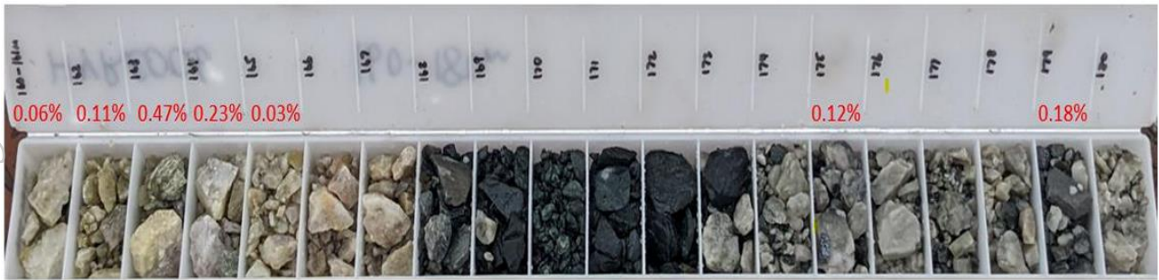
Figure 8: RC chips for 140-160m in HYRC006 with significant Li 2 O assays labelled in red
