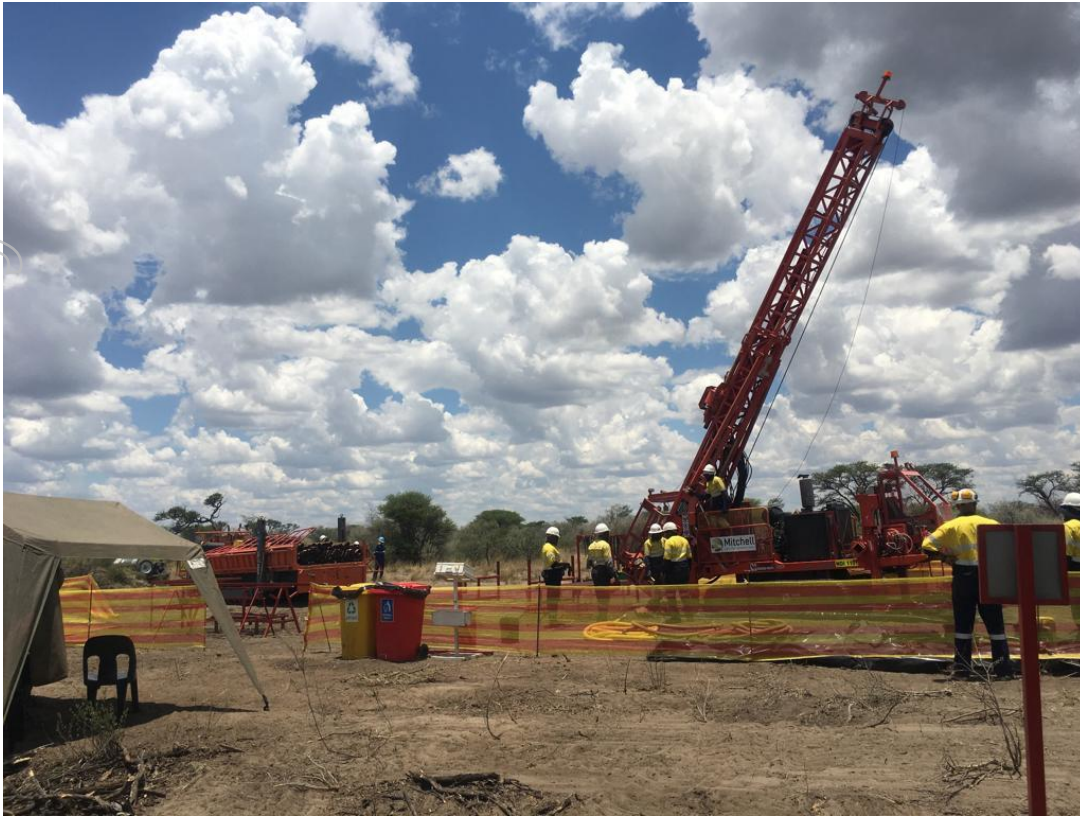
Figure 8: Diamond drilling underway at the Helm prospect, Snowball JV
