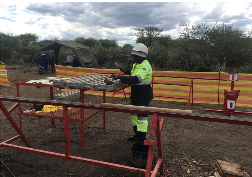
Figure 9. Diamond core being processed on site at 22HED01
