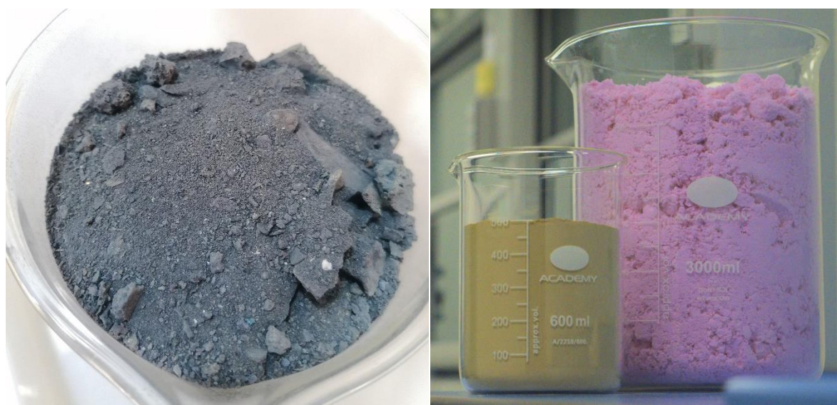
Figure 5: Swarf feedstock on the left, sourced from NdFeB metal alloy production, rich in Nd and Dy only, prior to production of intermediate products on the right – mixed Nd/Dy oxide (brown) and mixed Nd/Dy oxalate (pink).
