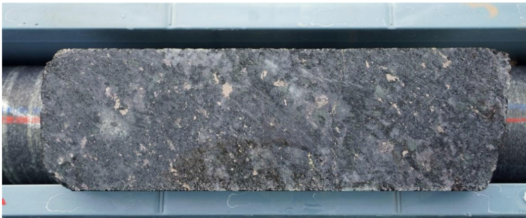
Figure Four | Disseminated sulphide bearing core from hole PS412
