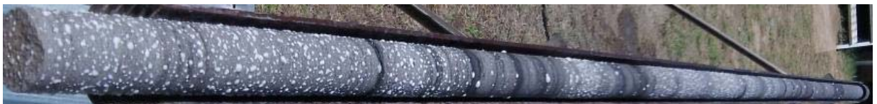
Figure 3: 3m core sample from 475m showing gassy sandstone formations
