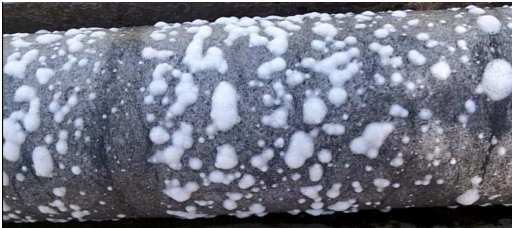
Figure 2: Core sample from 412m showing visible gas emissions using soapy water
