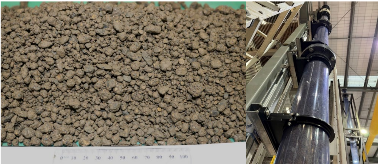
Figure 6: Agglomerates, post-curing, on the left, and a 5m heap desorption column under irrigation at ANSTO.
