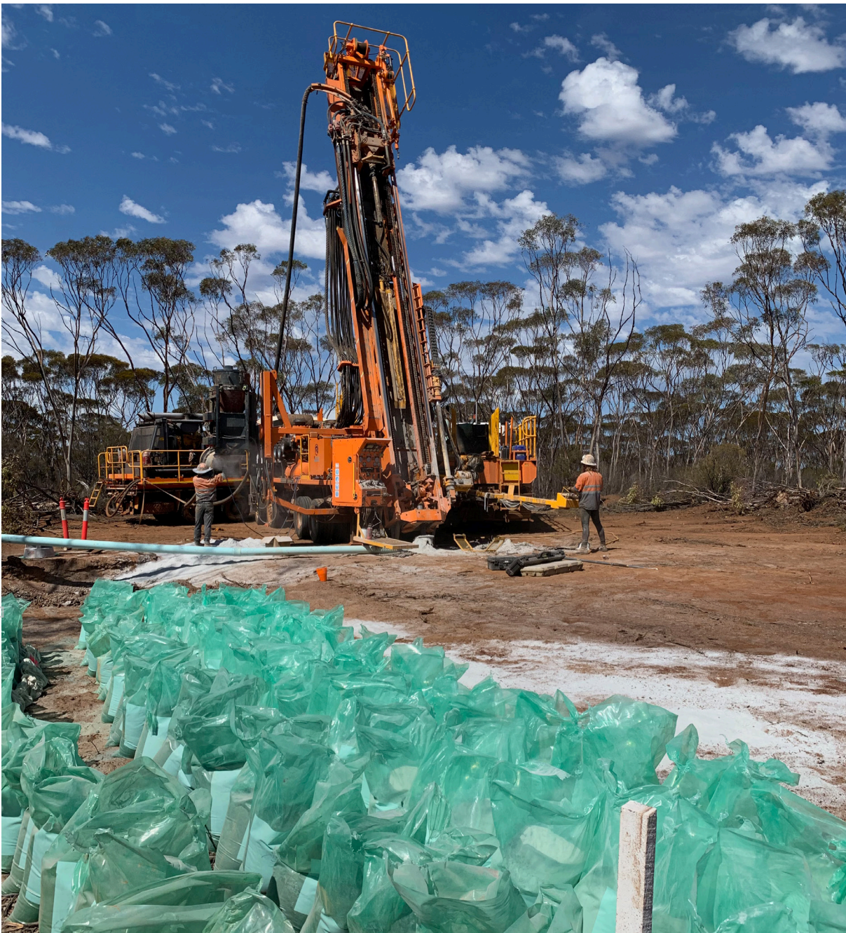
Photo 1 Reverse circulation drilling at Darson South – March 2023.
