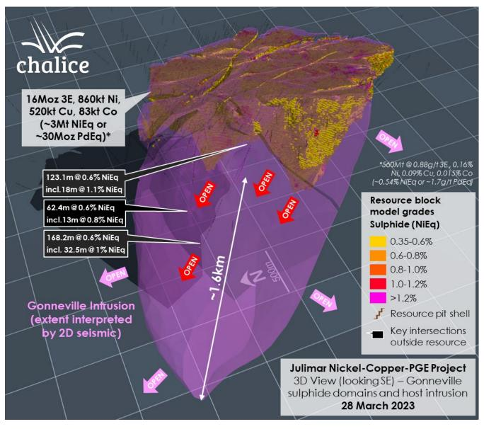
Figure 7. 3D view (looking SE) of Gonneville sulphide block model and host intrusion.
