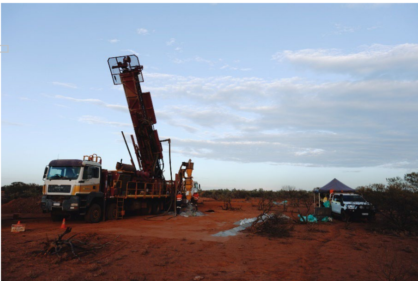
Figure 1: Photo of the RC rig drilling undercover ironstones to the south of the Yin Resource.
