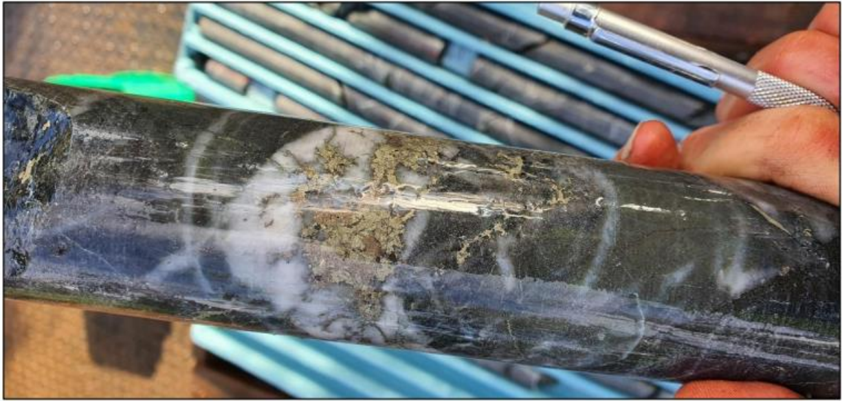
Figure 7: Chalcopyrite + Pyrite + Quartz veins from Hole 4 @ 322.5m
