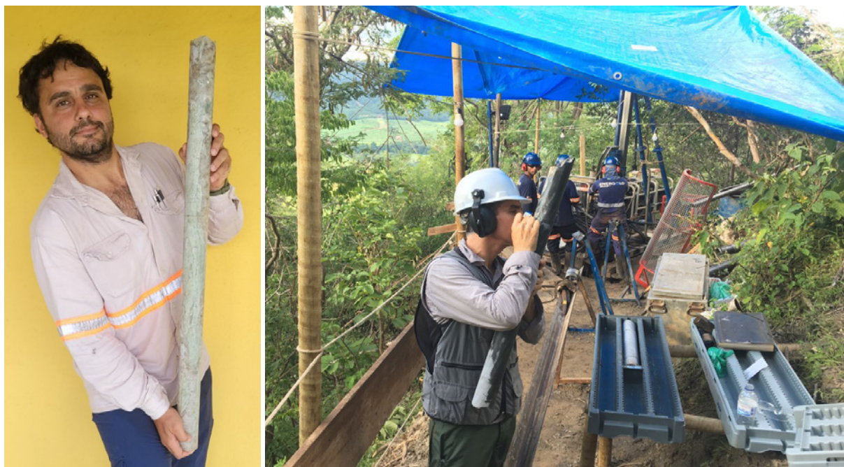
Figure 2: Salinas Lithium Project – Latin Resources Senior Geologist with spodumene rich pegmatite core, and core logging on site
