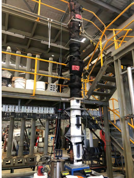
Image 11 | Nifty 6m high metallurgical test work column
