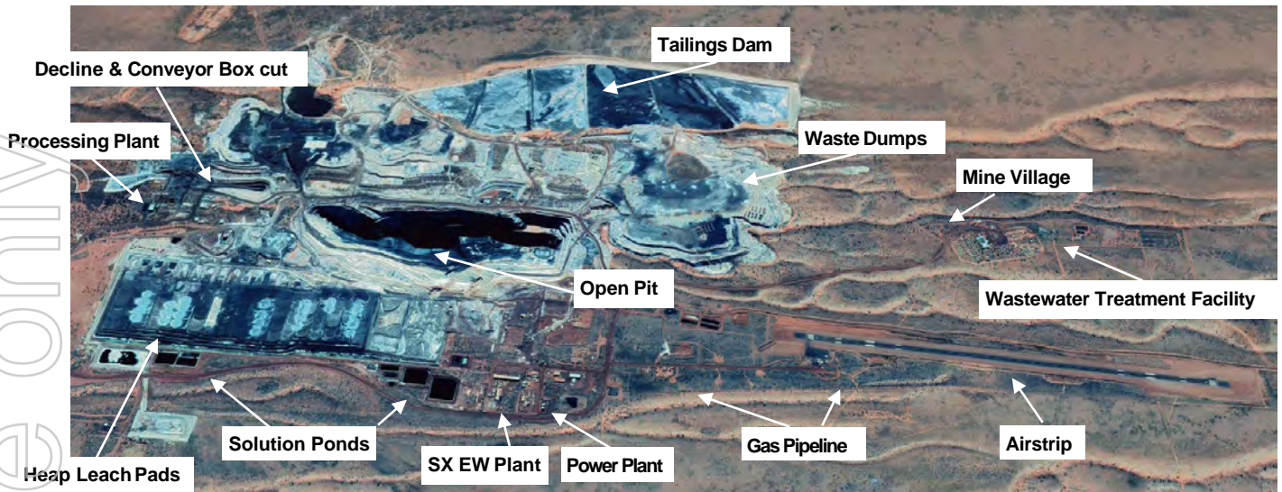
Figure 6 / Nifty Copper Mine Site Layout
