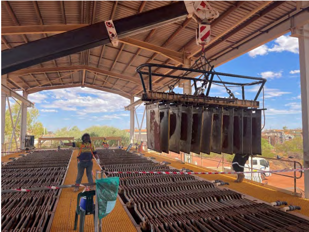
Image 2 / EW - Removal of Cathodes
