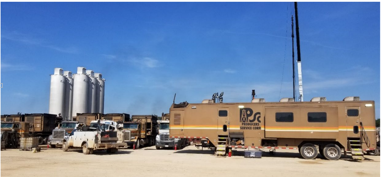
Figure 8. Producers Service Corp. (PSC) conducting multi-stage hydraulic stimulation operations on the Flames Well, Carter County, Oklahoma.
