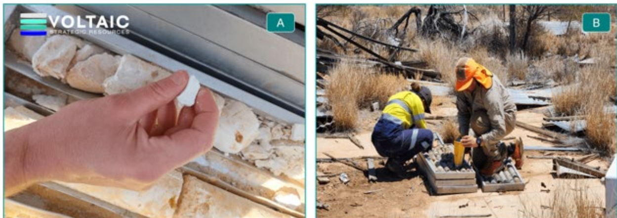
Figure 6: (a) Section of historical core with elevated REEs within kaolinite clay horizon, (b) Voltaic's team confirming REE anomalism utilising pXRF
