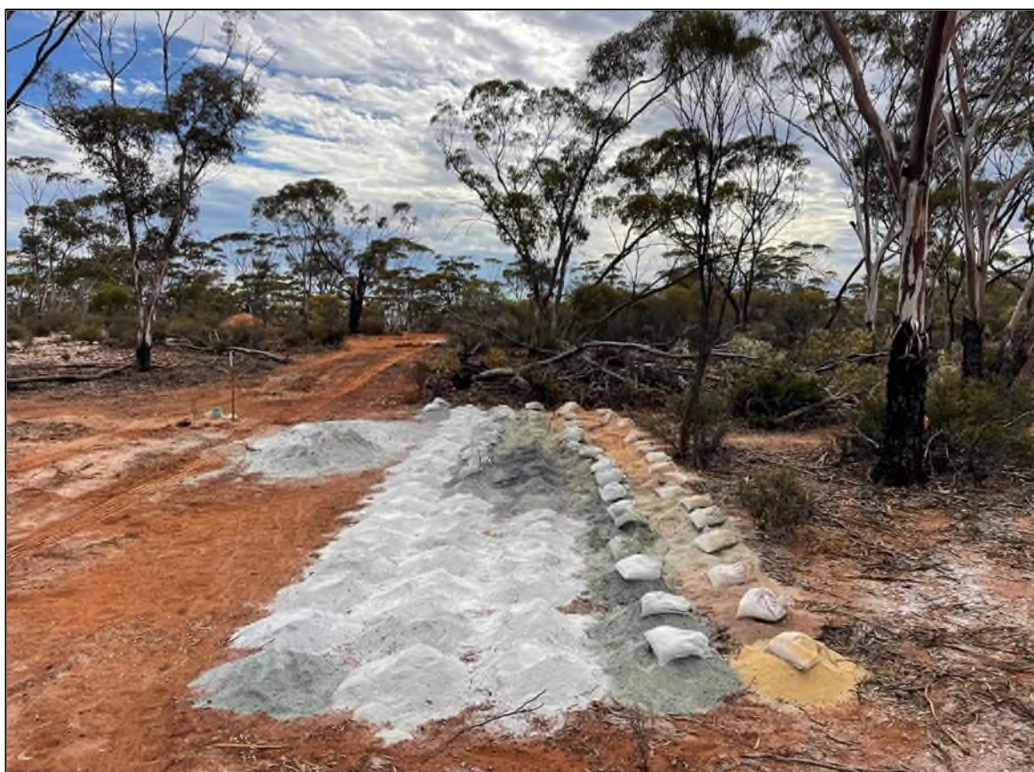
Figure 5 Drill spoils from hole 23RC031 showing wide zone of pegmatite (white samples)
