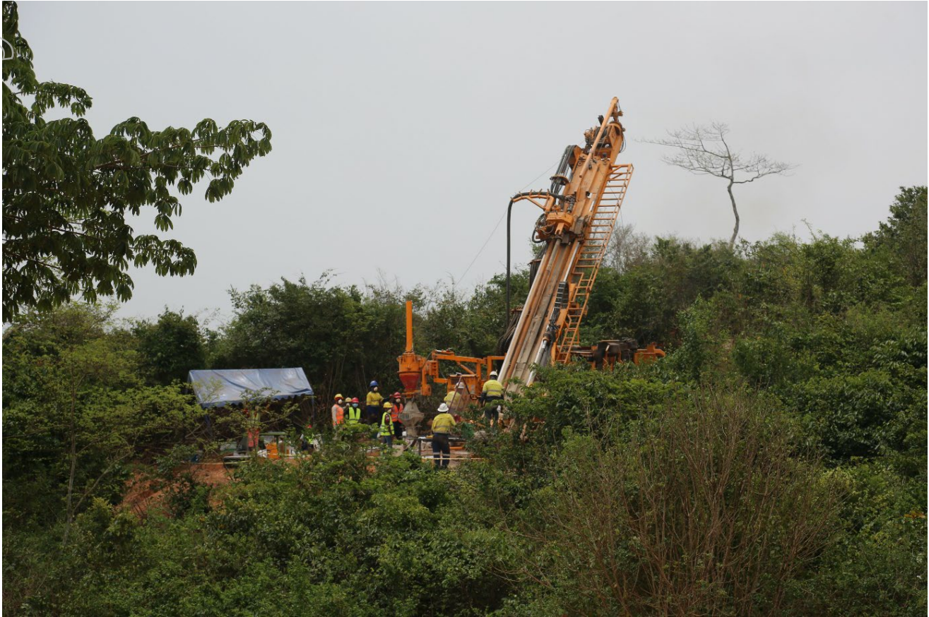
Infill drilling underway at the Ewoyaa South 2 deposit
