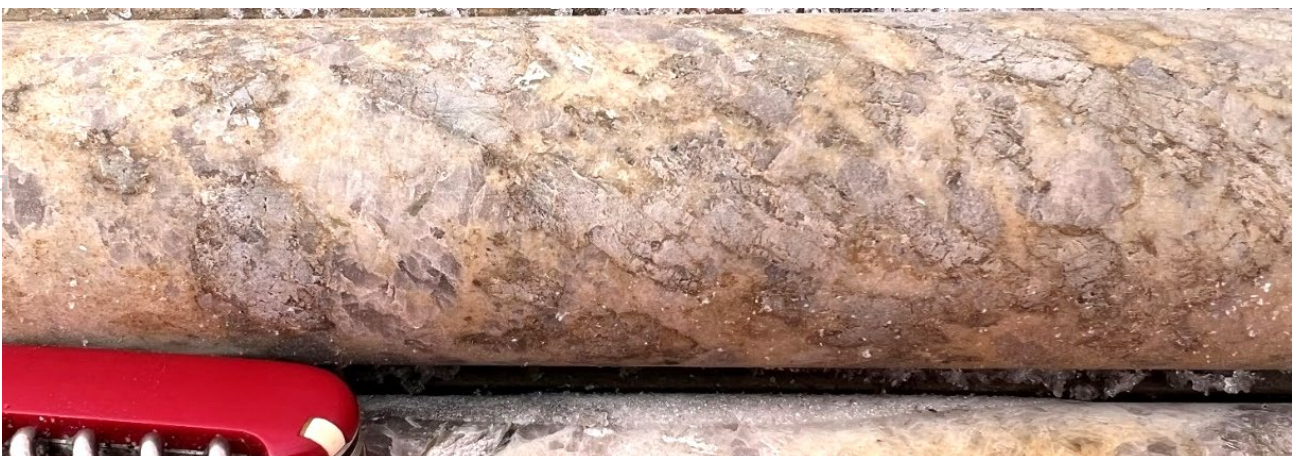
Figure 5: Visible spodumene* observed in drillcore from AC-2010-004 between 212.8m and 223.8m. 1 No historic drill core has ever been assayed for lithium bearing minerals.
