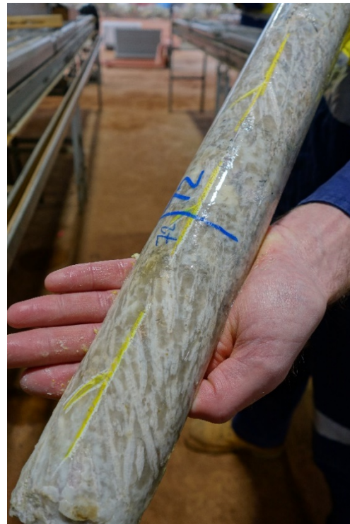
Figure 3 - Hole 1 (FFLIDD2301) core showing abundant coarse spodumene crystals
