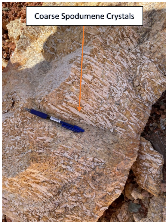
Figure 2 - Federal Flag Prospect – oxidised LCT pegmatite outcrop in old gold workings showing abundant coarse spodumene crystals
