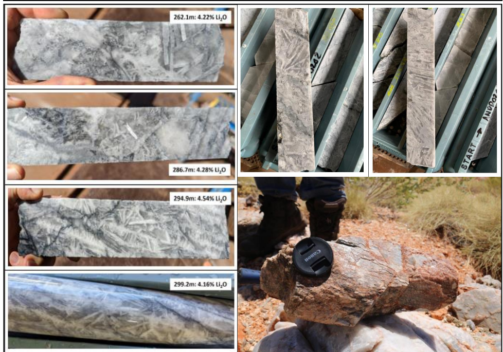
Figure 28: Coarse-bladed spodumene samples from Andover
