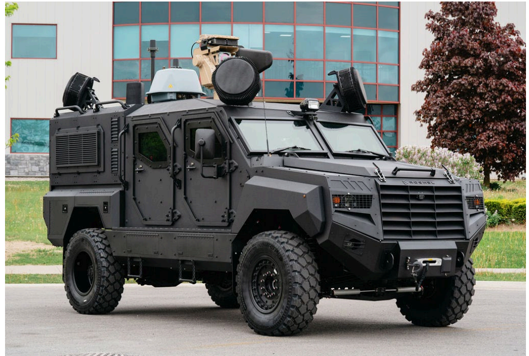
Image: Counter-UAS vehicle, featuring DroneShield's DroneSentry-X Mk2
