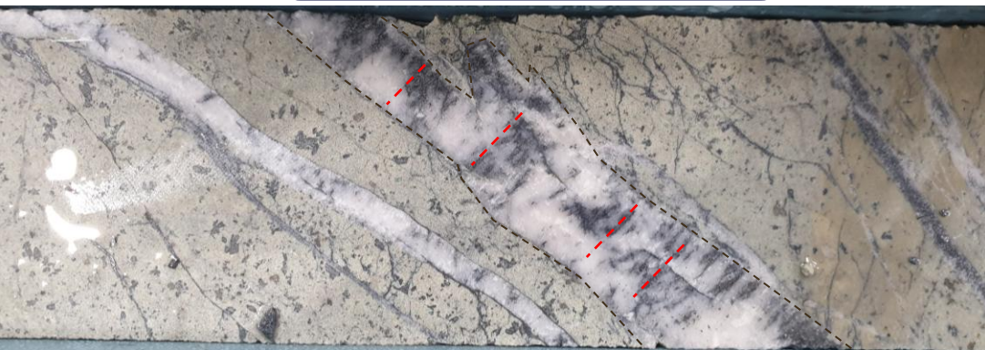
Quartz-carbonate-stibnite extension veins in altered dyke
